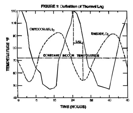
Masonry wall exhibit overall thermal performance superior to that of walls with metal framing systems with insulation of the same RSI value because their mass gives masonry walls the following advantages:
